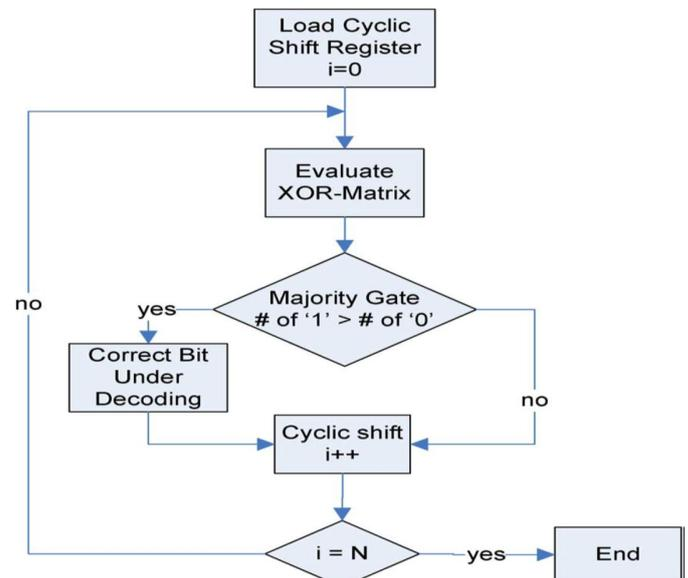
**Fig. 3. Flowchart of the ML algorithm.**
