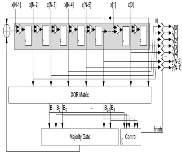
Fig. 6. Schematic of the proposed MLDD. i) Control unit. ii) Output tristate buffers.
