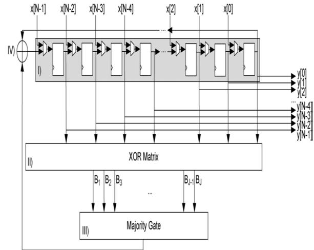
**Fig. 2. Schematic of an ML decoder. I) cyclic shift register. II) XOR matrix. III) Majority gate. IV) XOR for correction.**
