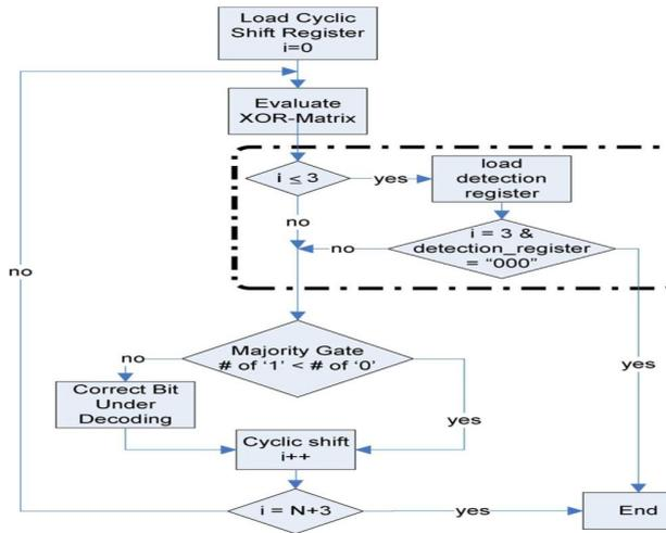
Fig. 5. Flow diagram of the MLDD algorithm.
