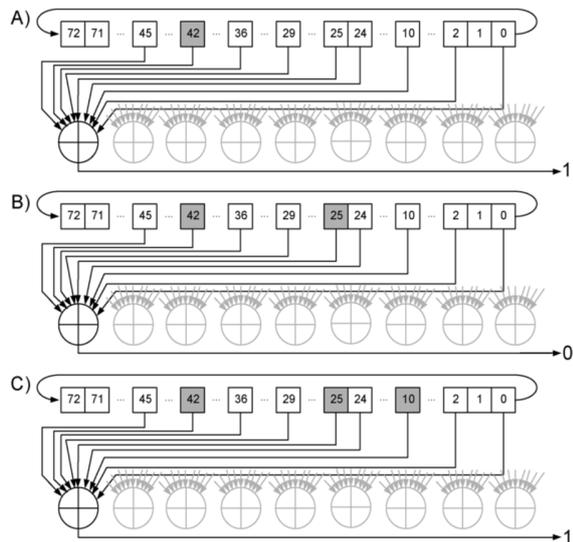
**Fig. 4. Single check equation of a ML decoder. (a) One bit-flip. (b) Two bit-flips. (c) Three bit-flips.**
